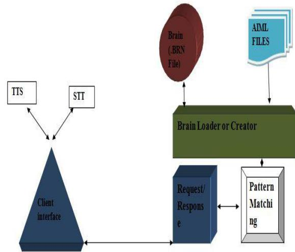
Fig. 4. Flow Diagram of Request and Response
