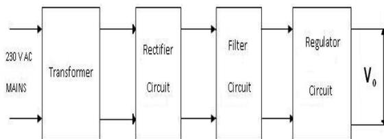
Fig.4.1.1. Power supply system
