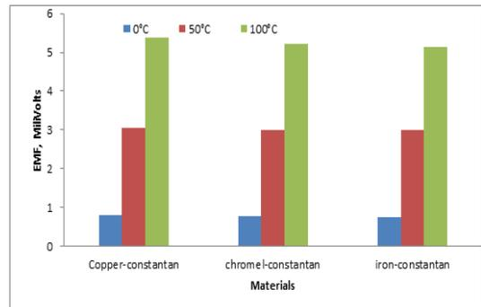
Fig. 2 Effect of change in temperature on EMF induced
