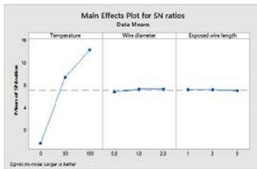
Fig. 6 Main effect plots for Chromel Constantan Thermocouple
