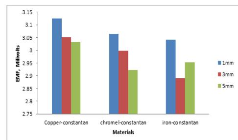
Fig. 4 Effect of Exposed wire length on EMF induced
