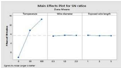
Fig. 5 Main effect plots for Copper-constantan Thermocouple
