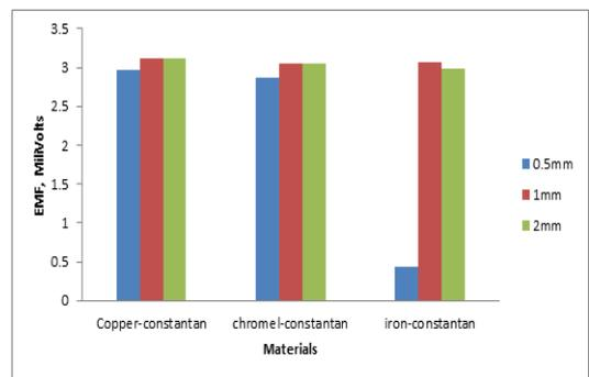
Fig. 3 Effect of Wire diameter on EMF induced
