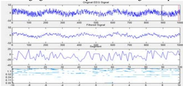
Fig 8. Original and Pre-processed signal of normal stage of sleep and corresponding SST
