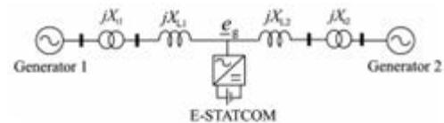
Fig. 1. Simplified two-machine system with E-STATCOM.
