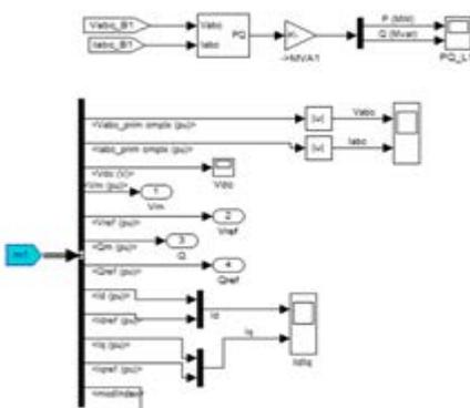
Fig 4.2 Simulink model of E-STATCOM.
