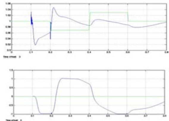
Fig 4.2.2 Measured Generator Power Output For Three-Phase Fault With E-Statcom
