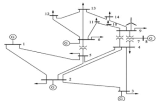
Fig: WPG connected at bus No. 9 (modified IEEE 14 bus system).
