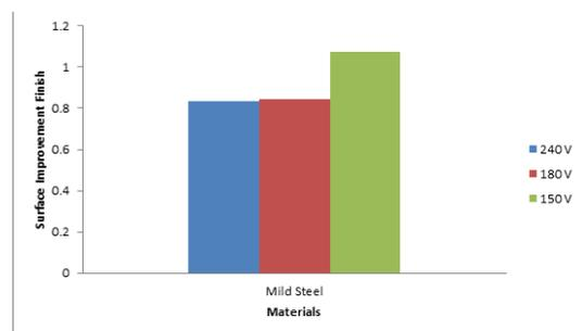
Figure 3. Effect of Voltage on Surface roughness improvement
