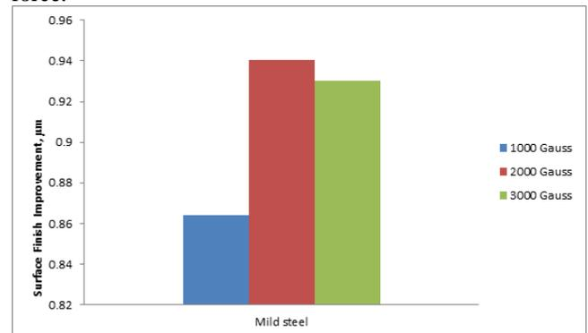
Figure 2. Effect of change in magnetic flux density on Magnetic abrasive machining
