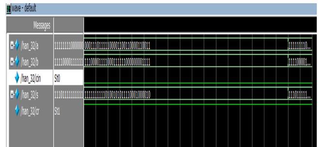
Fig.5.1 Simulation result of 32\*32 bit Vedic multiplier
