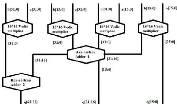
Fig.4.1 Block Diagram of proposed method using Han-Carlson
