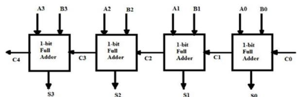
Fig.1.1 Block Diagram of Ripple Carry Adder
