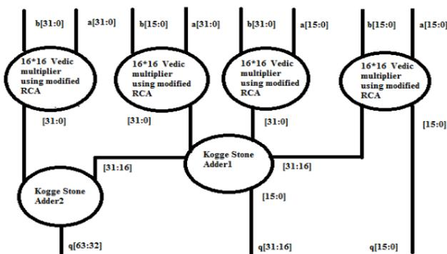
Fig.3.1 Block Diagram of existing 32\*32 bit vedic multiplier
