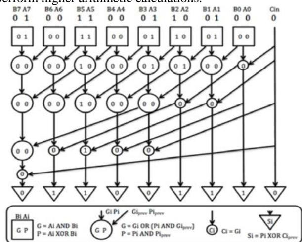
Fig.2.1 Block Diagram of Kogge Stone Adder.
