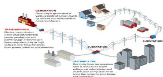
Fig 1: Distribution of electricity from generating station to consumer end
