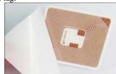
Fig 5: RFID tag showing microchip
