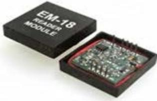
Fig 6: RFID reader module.
