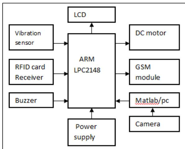
Fig 2: Block diagram of ATC.
