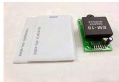
Fig 4 : RFID tag and Reader.
