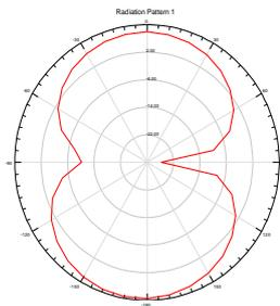
Fig.10(a): E-plane and H-plane patterns at 5.80 GHz
