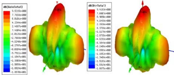
Fig.9(b):Gain and Directivity at 8.92 GHz
