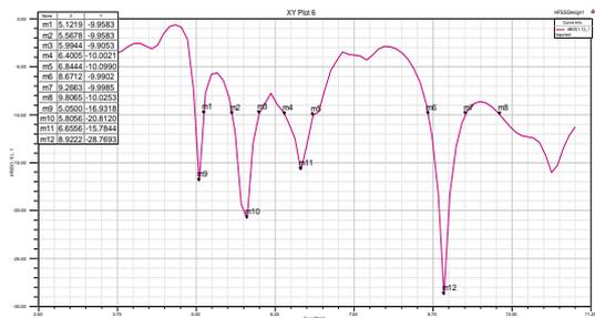
Fig. 8. Return loss curve with dual notch band
