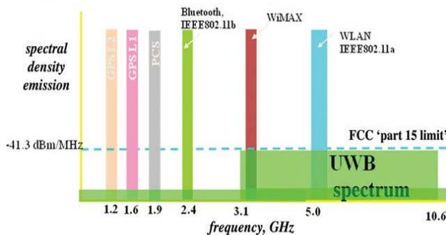
Fig.1:Coexistence of various wireless systems with UWB band
