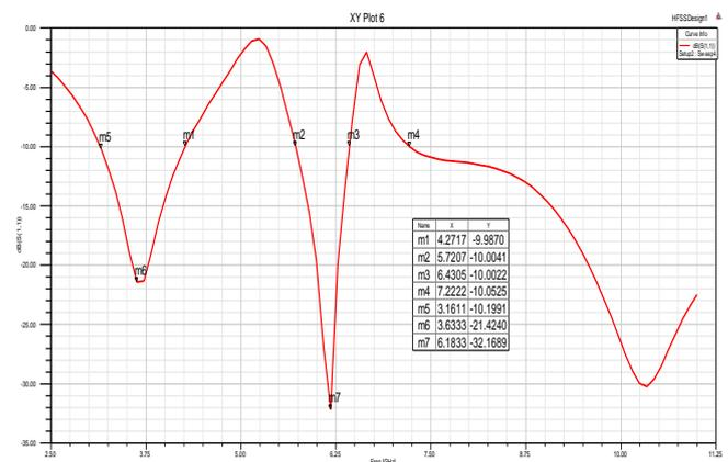
Fig4: Return loss curve with dual notch band
