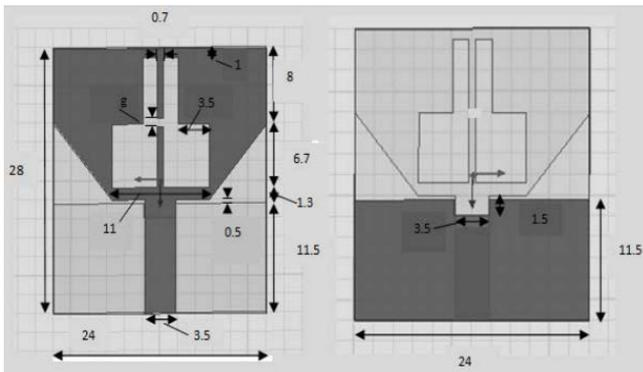
Fig. 2: Proposed design: Top view and bottom view
