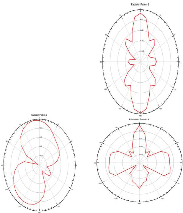
Fig.10(b): E-plane and H-plane patterns at 8.92 GHz
