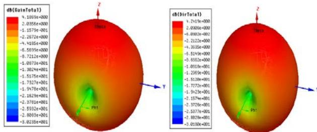
Fig.5(b): Gain and Directivity at 6.18 GHz
