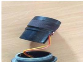
In the magneto-dynamic microphone, a thin metal diaphragm and a wire coil attached to it vibrates (to-fro movement) due to the incoming sound waves. A magnetic field round the coil is thus caused which moves the scroll within this area. This in- turn causes current to flow. The velocity of the apparent movement of diaphragm determines the sum of current produced. This is a velocity sensitive microphone.
