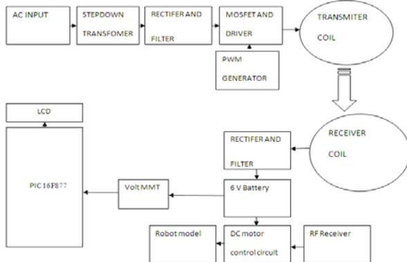
Fig 2: Wireless Power Transfer from road to electric vehicle
