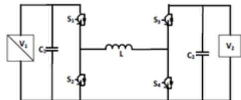
Fig.1: Cascaded Buck Boost Inductor in the middle (CBB-IIM)
