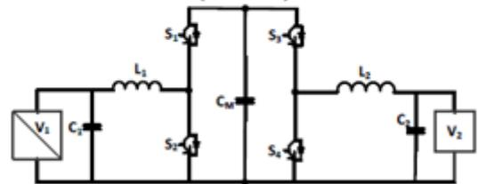
Fig.2: Cascaded Buck Boost Capacitor in the middle (CBB-CIM)
