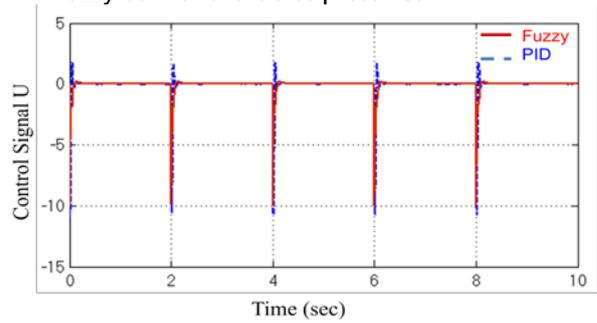
Figure 7Generated Control Signal from PID & Fuzzy controller It shows that the inverted pendulum system is unstable without the controller. Put the controller gain to design the simulation program in the Simulink environment. The results of the control signal for PID & Fuzzy controller for inverted pendulum system are shown in Figure 7.
