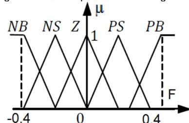
Figure 5 Membership function for actuator force
