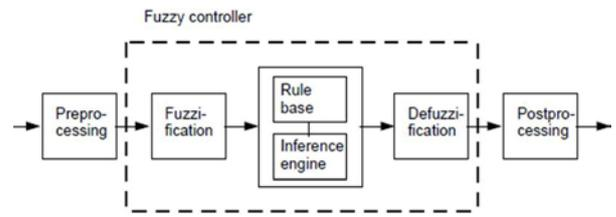
Figure 2 layout of fuzzy logic control
