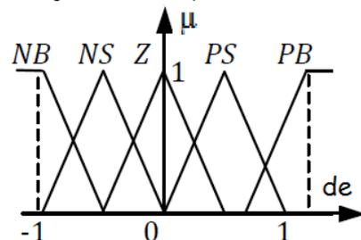
Figure 4 Membership function for change in error
