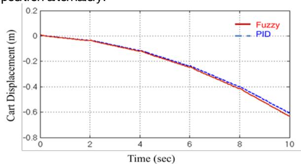
Figure 9 Displacement of Cart for PID & Fuzzy controller In this case, Fuzzy Logic controller takes less setting time than PID Controller. Simulation results show that the system responses converge to the equilibrium point,which indicates that the design of the fuzzy controller is stable.
