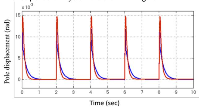
Fig.8Displacement of pole for PID & Fuzzy controller Initially, input disturbance force of square-wave signal is applied to cart. In Figures 8& 9, the initial angle of the pendulum is 0.015 rad and the other initial values are all zeros. It takes 1 sec for fuzzy controller to be stabilize pole on cart, whereas PID controller takes 1.3 sec.The pendulum system is managed to be stabilized in upright position, even though the disturbance is applied to the cart position alternately.
