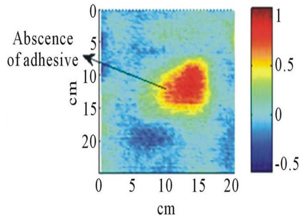
Fig.9. Thermal contrast between the specimen in the absence of adhesive
