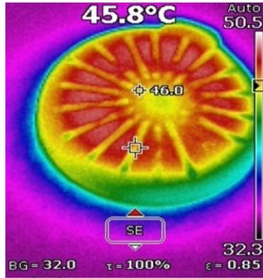
Fig.3. Thermography image of nitrile rubber
