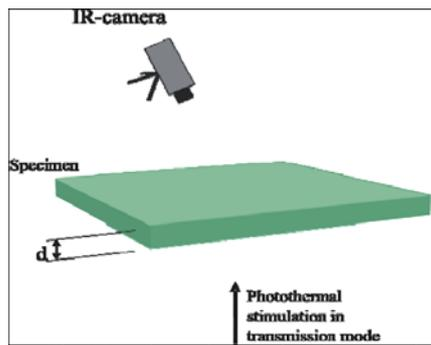
Fig.1. Experimental setup of IR thermography
