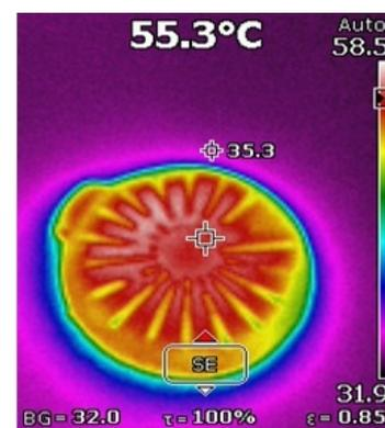
Fig.2. Thermography image of Butyl rubber
