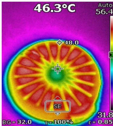
Fig.4. Thermography image of fluoro-silicone rubber
