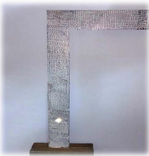
Fig. 1. Fabricated model of L-shape beam
