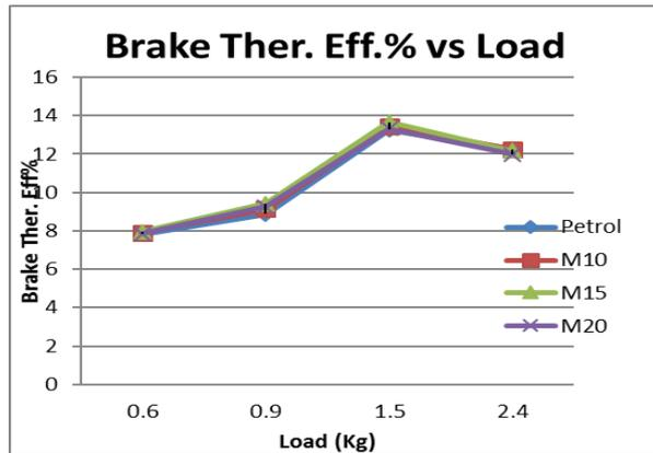
Fig.3 Brake Thermal Efficiency vs Load
