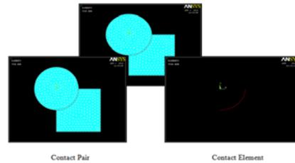
The problem is treated as thermal contact problem so its must to create a contact pair between the contaminated particle and the bearing surface. The target surface is bearing surface and the contact surface is a particle.
