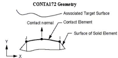
Contact 172 elements are created at the surface contact between the target and the contact surface. The contact properties and the boundary conditions, thermal loads are given as input to carry out the contact analysis in order to find the flash temperature at the contact region.
