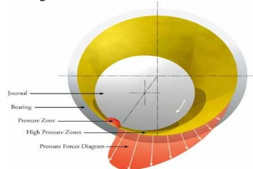
However, it is equally important to consider particle size and the fluid cleanliness level required for journal bearing operation. Removal of clearance-sized particles is required for wear reduction and scuffing failure, and can be achieved by implementing high efficiency filtration to lubrication systems equipped with journal bearings.
