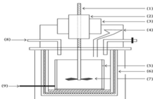
(1) Stirrer spindle, (2) sliding mechanism with impeller position control unit, (3) electric motor, (4) sprue, (5) crucible, (6) electric furnace, (7) impeller, (8) argon gas inlet, and (9) Thermocouple.
