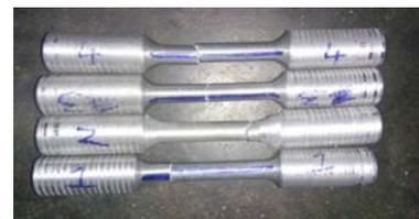
Figure 7 Tensile test specimens
