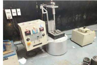
Figure 5 Conventional Stir casting machine with preheater.
