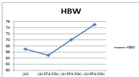
Figure 10 Comparison of hardness results
