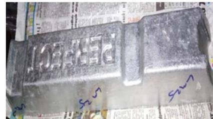
Figure 1 Aluminium lm25 ingot
