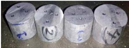
Figure 9 Hardness test specimens
