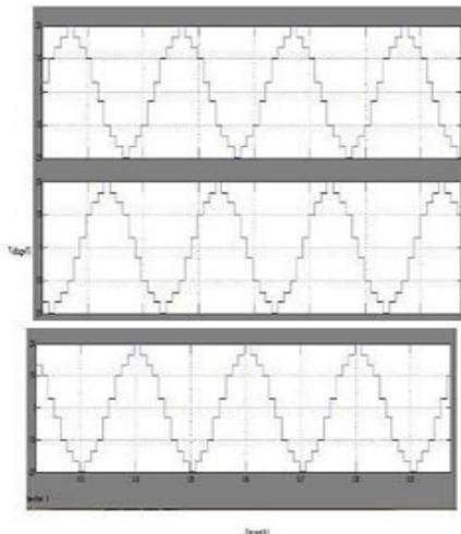
Fig: 3 Phase voltage of 11 Switch Three Phase Multilevel Inverter
