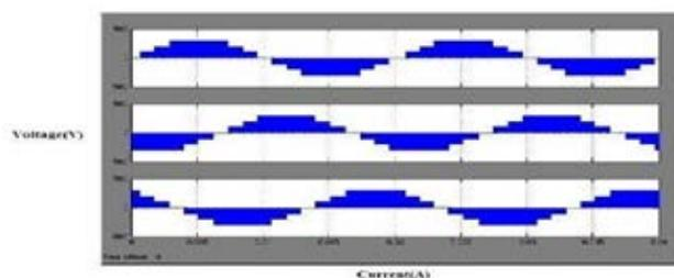
Fig: 6 Phase voltage of 11 Switch Three Phase Multilevel Inverter using PWM
