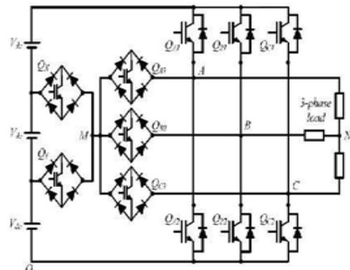
Fig: 1 The proposed multilevel inverter circuit topology
