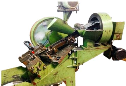
Fig.2 Conventional Bolt Feeder Machine or Rotary Feeder Machine
