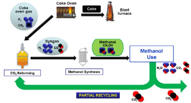
Fig 2: Partial recycling of by mean of reforming of coke oven gas for methanol production.
