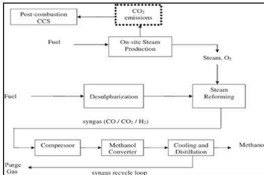
Fig. 1. The flow chart of the methanol synthesis process [16].
