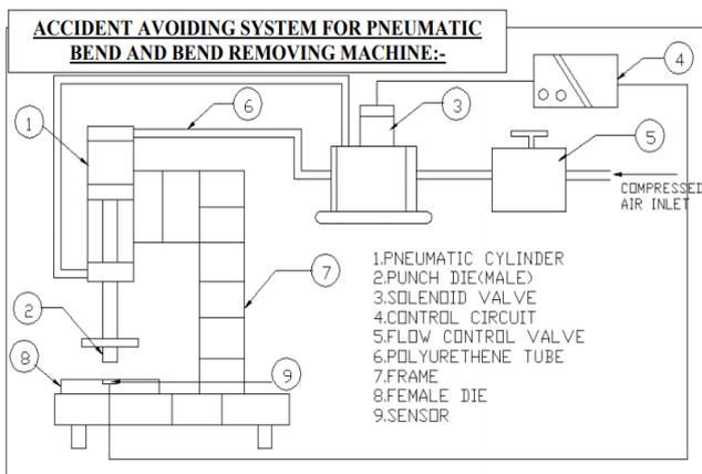
**Fig. 2 – Construction diagram**
